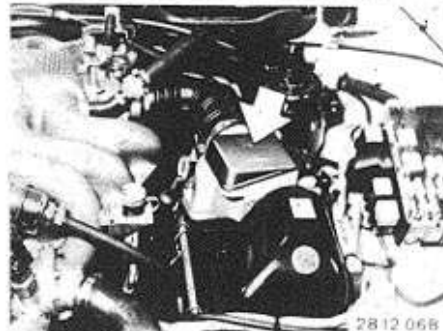
Air flow sensor (air temperature sensor is integrated in air flow sensor)
