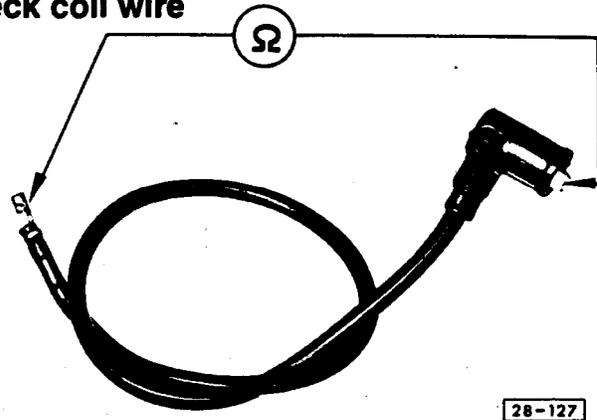
Coil wire resistance should be 800 to 1200 ohms.
