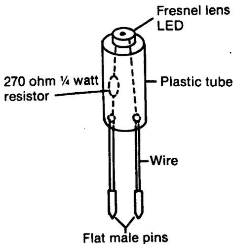
An LED is used to check the low voltage signal from the reference mark and speed sensors. One of these testers will be sent to every dealer. The tester, however can be made from locally available components which are available at Radio Shack or any other electronics store.
