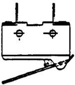
Remove wire from idle switch
