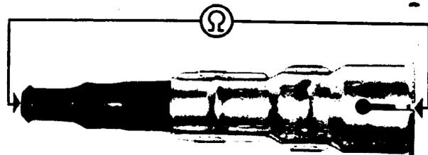
Connector resistance should be 4000 to 6000 ohms.
