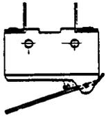
Trip full throttle switch (engine at idle so idle sw. is closed).
