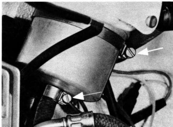
DEPOSE ET REPOSE DE L'ACCUMULATEUR D'ESSENCE
